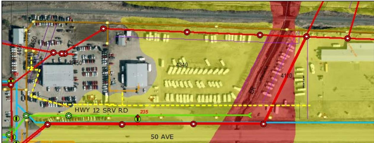
The gas line, as shown in yellow, will need to be protected by a Utility Right of Way. The remaining infrastructure will not be affected by the Road Closure.
